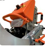
Double motors feeding system with speed control
